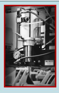
Blade Tension by Air and Hydraulic Compensation System to ensure a constant blade tensión at all time.
